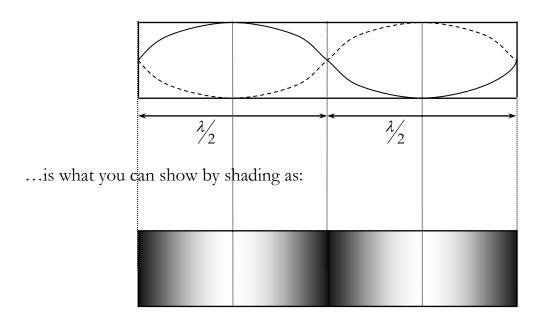
Using the idea of a wave-shape also makes it easier to understand where the half- and quarter-wavelengths fit into the pipe, as shown above.
