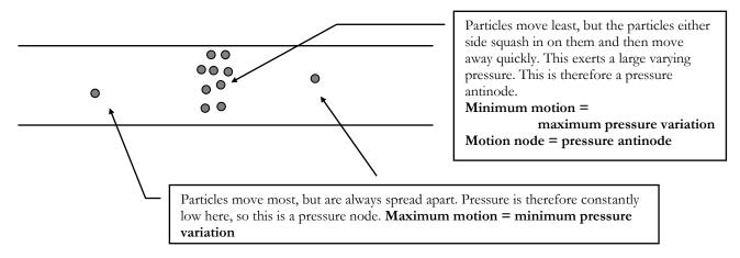
In the experiment with powder in a tube and a loudspeaker to create a standing wave (Kundt's Tube) the powder collects in areas of minimum particle motion (*i.e.* motion nodes/pressure antinodes).
