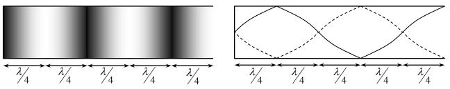
As you can see, with this type of tube, you always get an **odd** number of **quarter**-wavelengths fitting into the tube, whatever the frequency of the standing wave.
